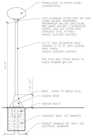
5 NEW LIGHT FIXTURE, TYPE A DETAIL
