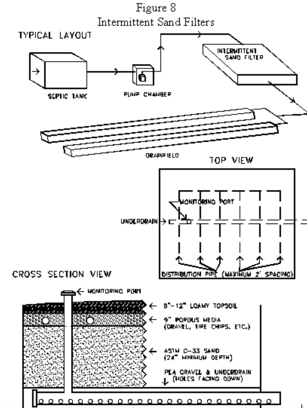
(9) Figure 9. Intermittent Sand Filter Underdrain and Pumpwell.
