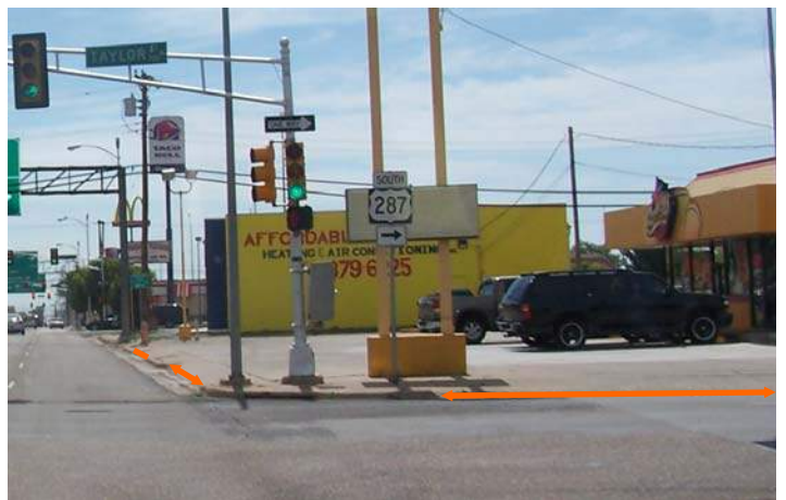
This example shows the extent of access (orange) that was permitted for earlier site development, even for a corner property at the intersection of two major highways (Bus. 40 and U.S. 287).
