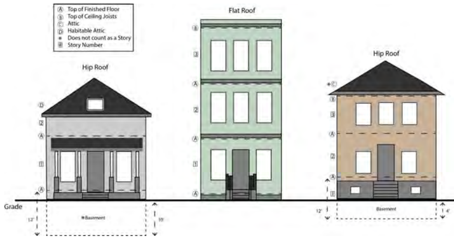
Figure 4-10-445277.1 – Measurement of Height in Stories
