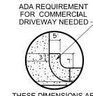
THESE DIMENSIONS ARE BASED UPON THE MIN, 10 FT. RADIUS AND 6 FT. COMMERCIAL SIDEWALK. THEY WILL VARY FOR LARGER RADII.
