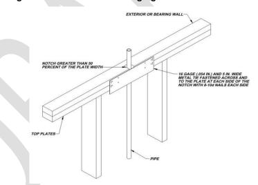
(Amendment to 2015 IRC carried forward to 2018 IRC also provides additional assurance of maintaining the integrity of the framing by spreading the nailing pattern.)
