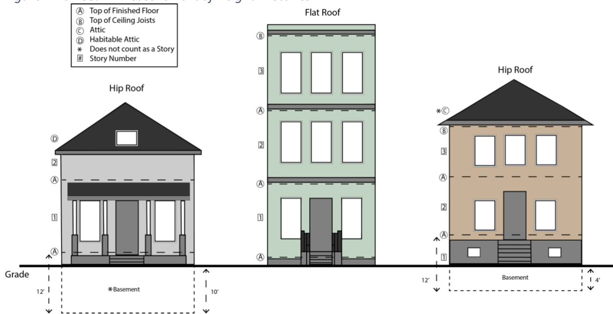
Figure 4-10-135.1 – Measurement of Height in Stories
