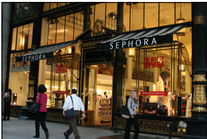
Awning and canopy signs are a good way to identify retail businesses. Awnings should be of quality material and relate to the shape of the window or door opening.
