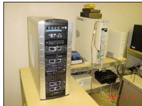
"Forensic Recovery of Evidence Device" = F.R.E.D
